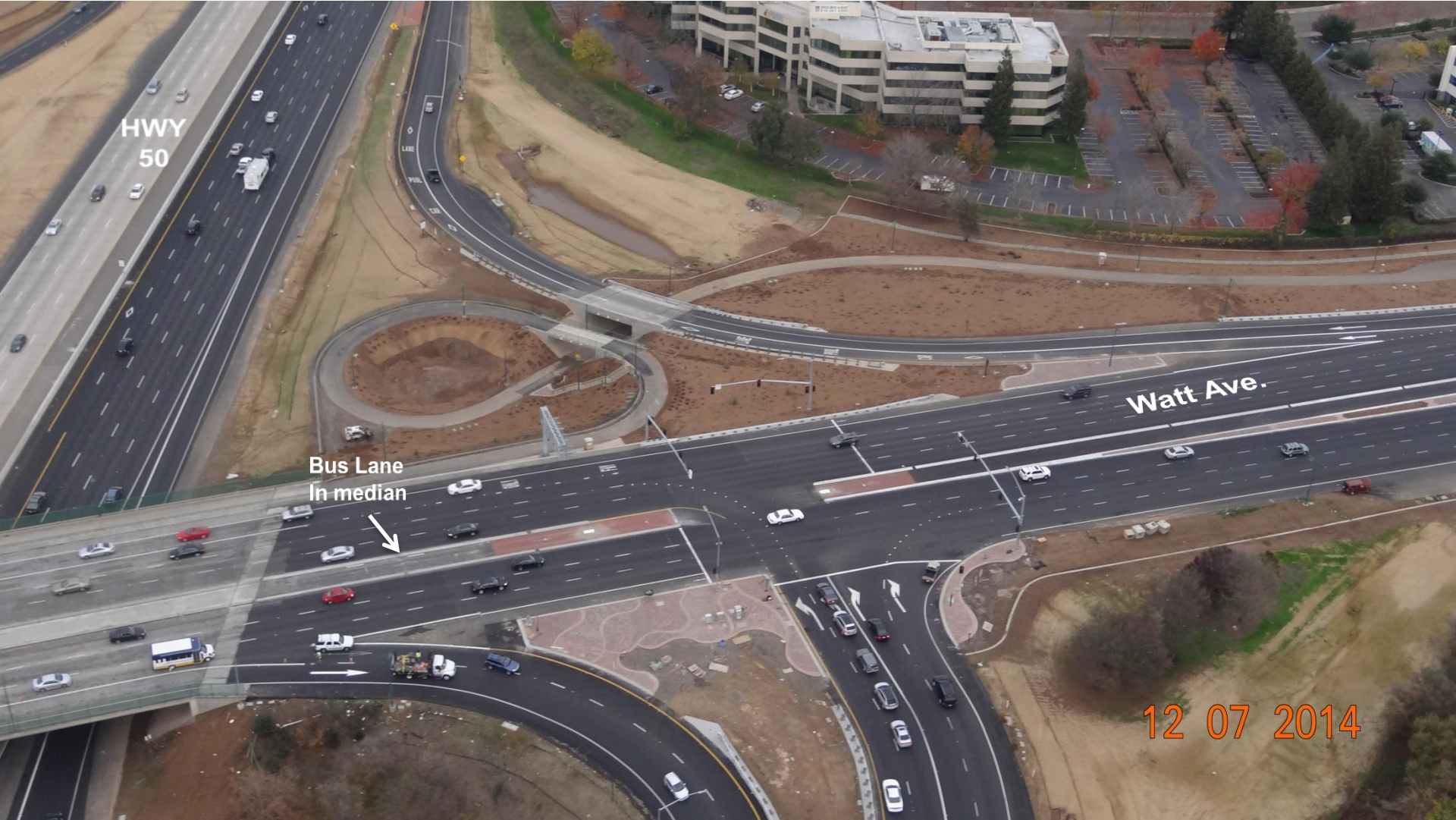
Watt Avenue at the interchange of eastbound US-50, facing east. On the right side of the photo, the exclusive bus lane can be seen in the median of Watt Avenue. A break in the bus lane allows cars to turn left from the eastbound US-50 off-ramp onto northbound Watt Avenue. The bus lane continues north on Watt Avenue in the median, with red pavement, a raised curb, and prominent signage helping keep general motorists out of the bus lane. The single bus lane would be shared by both northbound and southbound buses, with signaling and operating procedures developed to prevent occupancy of the lane by buses travelling in opposite directions (similar to a single-tracked rail segment).
